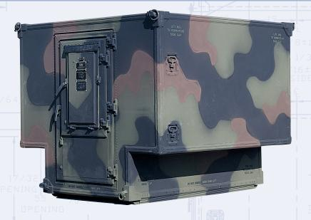
The S-250/G shelter makes it possible to transport and operate a wide variety of communications and electronics equipment to the field as a mobile unit. This high-strength, insulated, all-weather, general purpose mobile unit is designed to meet the user's specifications for complete systems integration.
